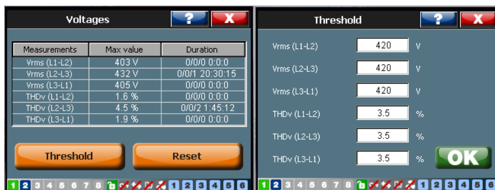
Figure 64: Example of the Min/Max logging function (4-W mode)
