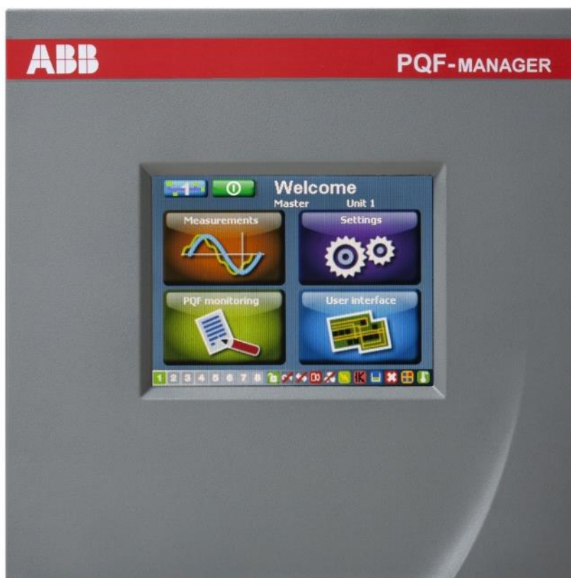
Figure 51: Front view of the PQF-Manager user interface
